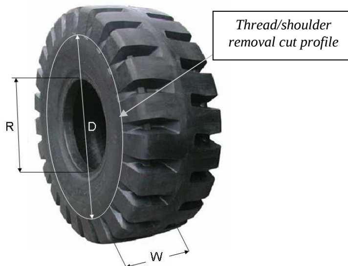
Figure 8 Pattern of separation cut with abrasive waterjet
