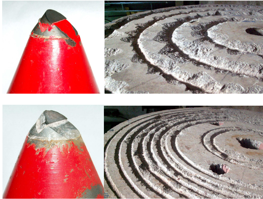
Figure 2. Grooves with new (top) and worn bit (bottom)
