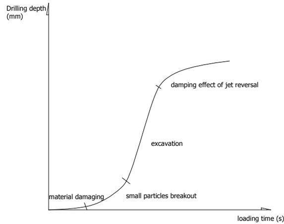
Figure 3 – Excavation model proposed by Erdman – Jesnitzer et al.
