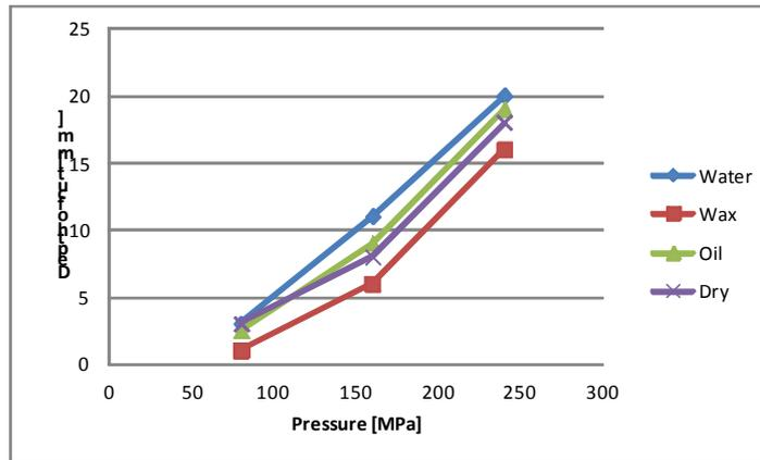
Figure 1- Depth of cut as a function of pressure for the different experimental conditions.
