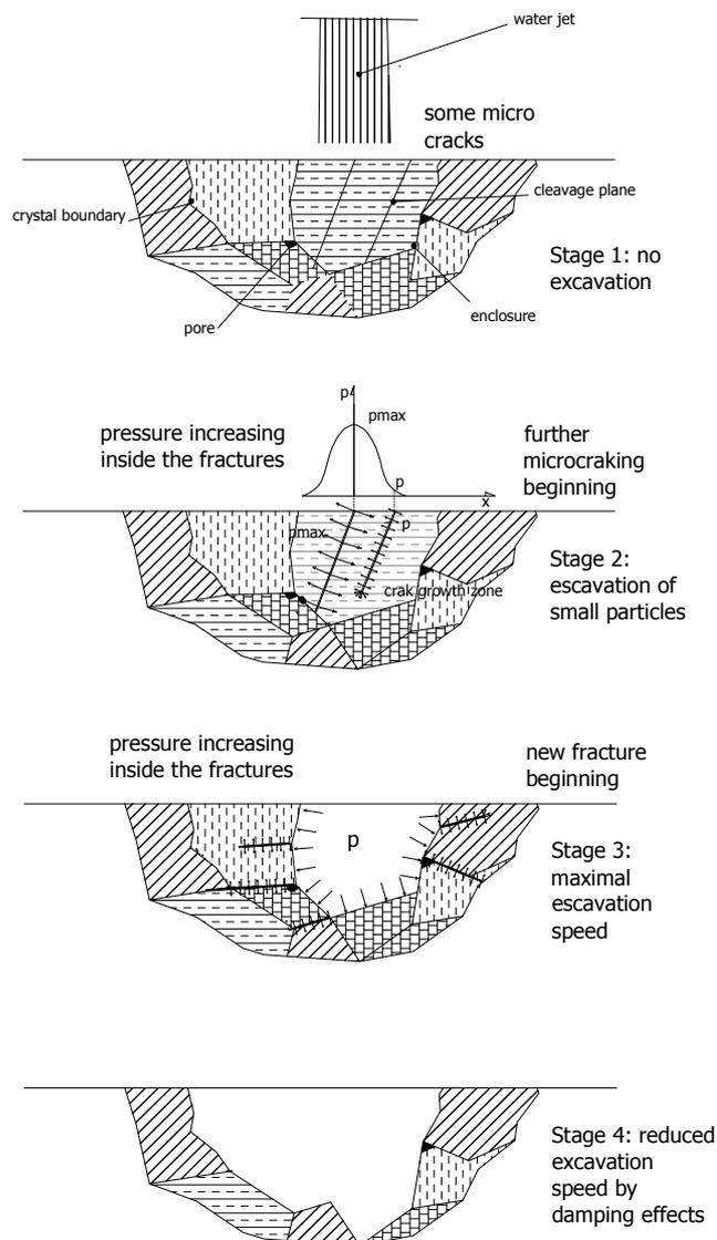
Figure 4 – Schematic representation of the new cutting model
