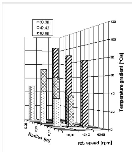
Figure 10. Tool's temperature raise measured with the thermocamera (top) at different experimental conditions.
