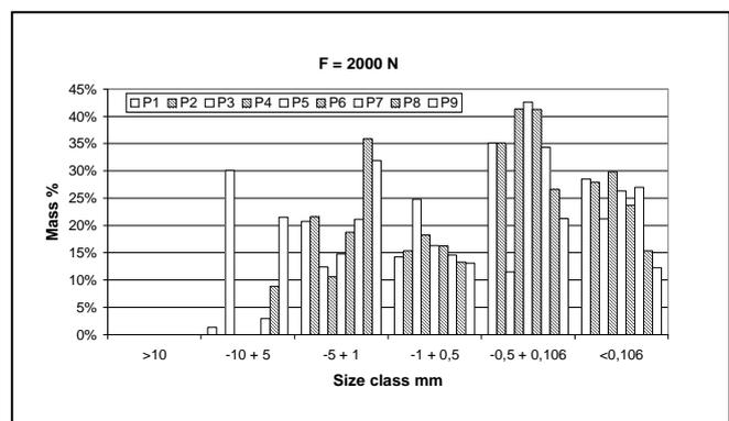
Figure 6. Results of excavation tests at 2.0 kN applied load (top) and corresponding size analysis of the cuttings.
