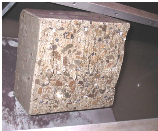
Figure 6. Appearance of the cut surface with the cutting strategy from both sides of the sample.
