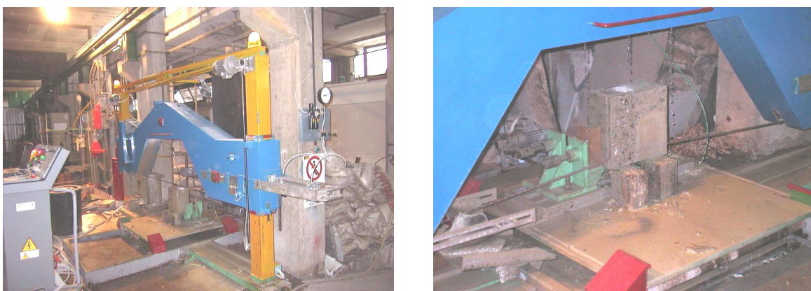
Figure 2. Overall view (left) and a detail (right) of the Diamond Wire cutting frame
