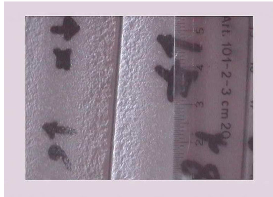
Figure 2. Typical zones of influence of the jet damage onto the stone surface
