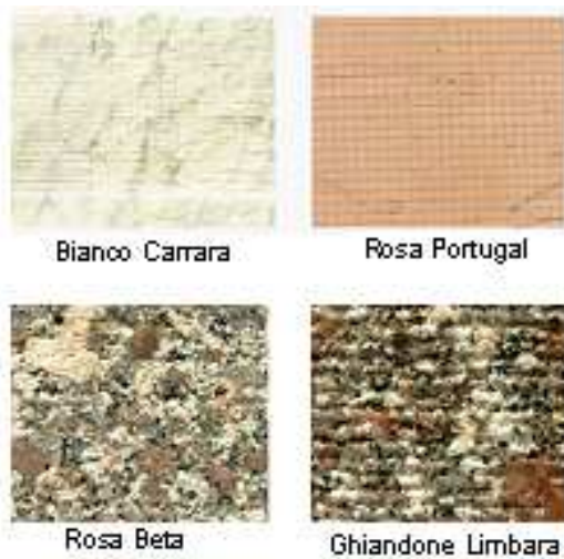
Figure 8. Results of surface finishing with plain waterjet on some granite and marble samples
