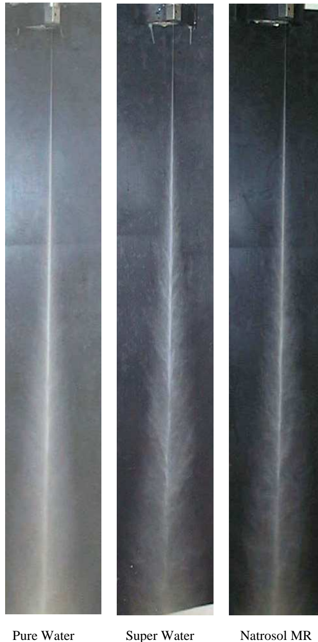
Figure 1. Features of water jets with or without polymer addition
